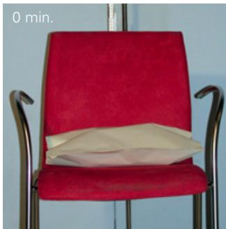
Test procedure according to DIN 66084 P-a
